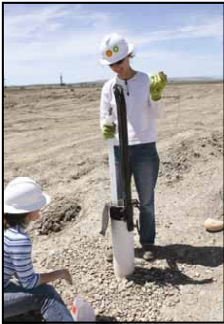
Above left: Samples being collected with polyethylene bailers. Above right: Samples being taken at an industrial water well with the aid of a pump.
